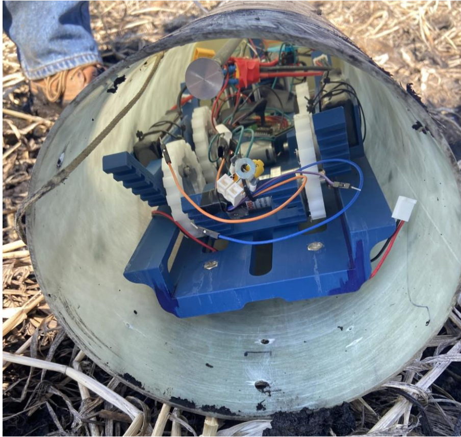
Figure 12: Payload system upon successful recovery and demonstration of orientation and retention system strength.
